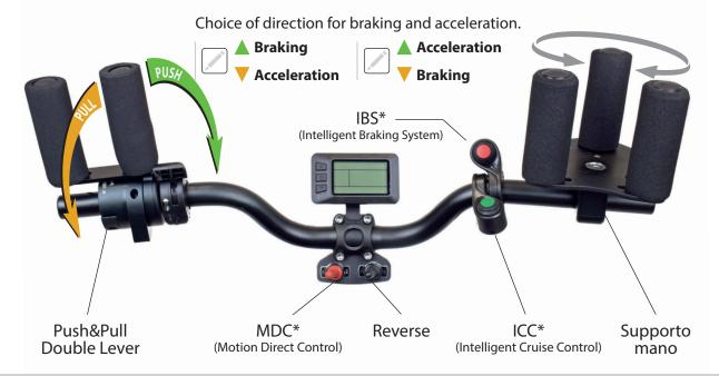
N.B. The triple hand turning supports function is to block the users wrist in order to drive and direct the Triride. The support is completely adjustable and customizable.
