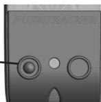
Once the power assist is turned ON [OLED displays “SD ON”] and the PushTracker is connected to the SmartDrive, the Indication LED will flash blue. When the SmartDrive motor is driving, the Indication LED will be solid blue. The Indication LED will flash red when the PushTracker is trying to connect or has lost wireless connection to the SmartDrive. Whenever there is a change of state to the SmartDrive, you will feel vibration as additional indication from the PushTracker.
